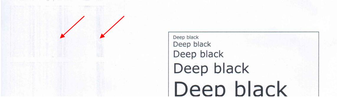
Waste streaks, as indicated by arrows above, are caused by complete filling of the cartridge's waste compartment. As a first line of defence, try shaking the cartridge from side to side to re-distribute the waste so that it no longer impacts onto the OPC drum.
